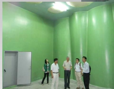
Photo 7: Reverberation room for testing acoustic panels
